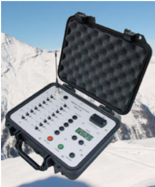
Figure 1. Barryvox Avalanche Training System, control box for up to 16 beacons.
