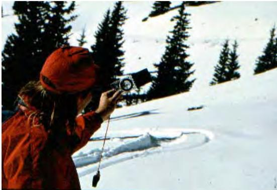
**Carrying an inclinometer helps measure slope angles. Photo: Ron Bookman**
