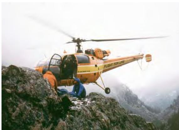
**For one-skid or hover boarding and exiting operations, extra caution must be used, and a few signals and procedures discussed beforehand with the pilot. Photo courtesy Flight for Life Colorado**
