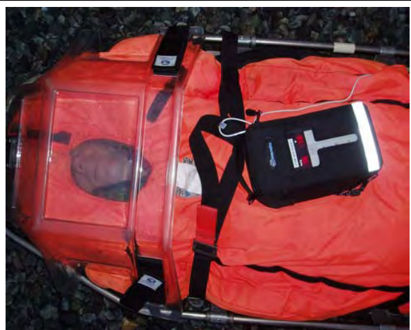
THE PULSE OXIMETER, DISPLAYING HEART RATE AND OXYGEN SATURATION, IS EASILY VISIBLE TO RESCUERS. THE MEASUREMENT PROBE IS TAPED TO A FINGER AND KEPT WARM INSIDE THE PATIENT PACKAGING. PHOTO BY STOWE MOUNTAIN RESCUE
