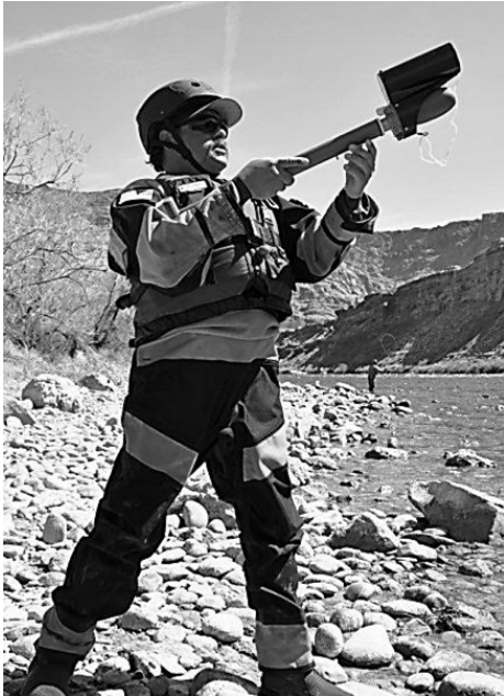
FIGURE 51. EZ Liner Line Launcher ready for use and positioned at an upward angle of 30 degrees.
