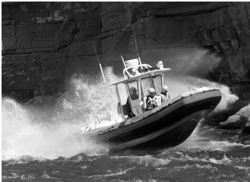
FIGURE 65. NPS 23-foot jet boat negotiates swiftwater on the Colorado River in Grand Canyon NP, below Lee's Ferry. The vessel has a 390-hp engine, which is powered a Hamilton 212 Jet Pump.
