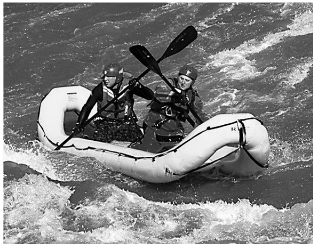
FIGURE 61. Oceanid Rapid Deployment Craft (RDC) is a hybrid watercraft that can be deployed in swiftwater responses. Image copyright Oceanid Inc. Reprinted with permission.
