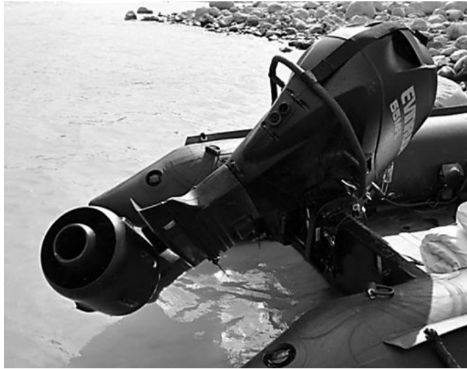
FIGURE 62. Evinrude 55-hp two-stroke multi-fuel outboard engine with a shrouded impeller, which handles submerged obstacles and is safe to operate around swimmers. Grand Canyon NP.
