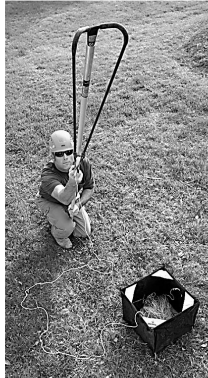
FIGURE 54. Sherill Big Shot Line Launcher. Image copyright Sherill Tree. Reprinted with permission.
