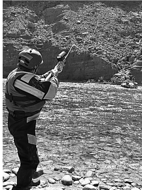
FIGURE 50. EZ Liner during successful deployment to a target 250 feet away.
