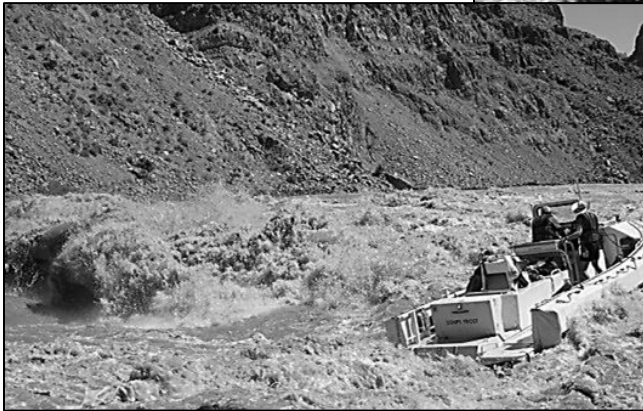
FIGURE 66. Canyonlands National Park jet boat in Cataract Canyon. A 450-hp diesel engine with a jet drive powers this 26-foot aluminum hulled vessel, which has a solid foam flotation collar.
