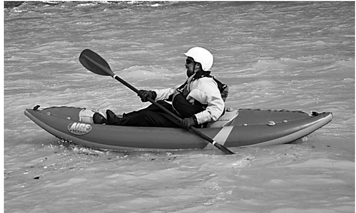
FIGURE 57. An inflatable kayak provides excellent mobility in swiftwater conditions and keeps the rescuer out of cold water. The AIRE Force model shown is 9' 6" in length and 36 inches wide. It has a load capacity of 275 lbs. and weighs 32 lbs. The tube diameter is 10.5" and contains four air chambers.
