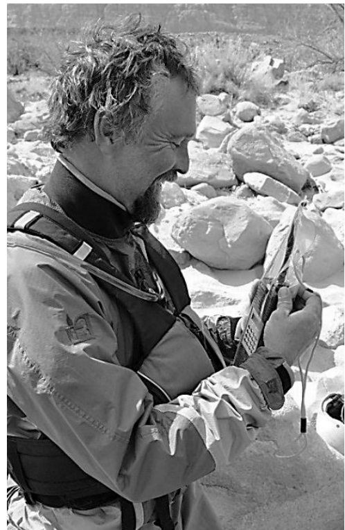
FIGURE 22. Preparing a handheld radio for use in a waterproof VHF radio case.
