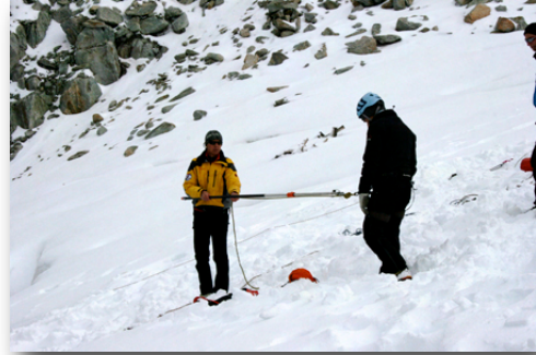
An adjustable length pole with a quick clip allows a rescuer to quickly attach a line to a stuck person.
