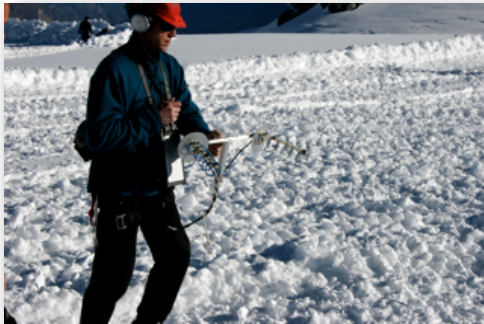
Hepkie ResQU mobile phone locator (does not show base station).
