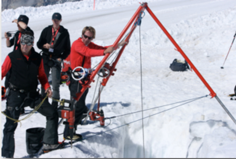
Jelk tripod, notice drill and chisel hanging from below the winches.
