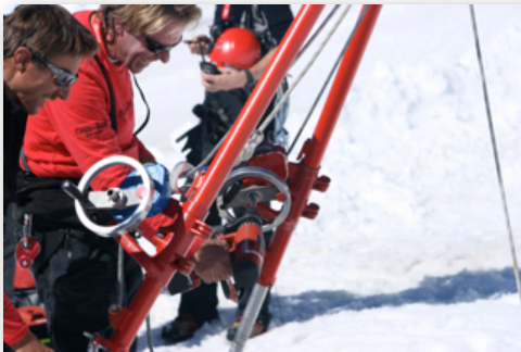
Electric drill used to power the winch.
