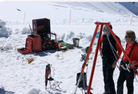
A gasoline-powered generator can be flown to the site to power the electric tools.
