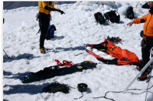
Kong litter system uses a carbon fiber backboard placed inside a casualty bag.
