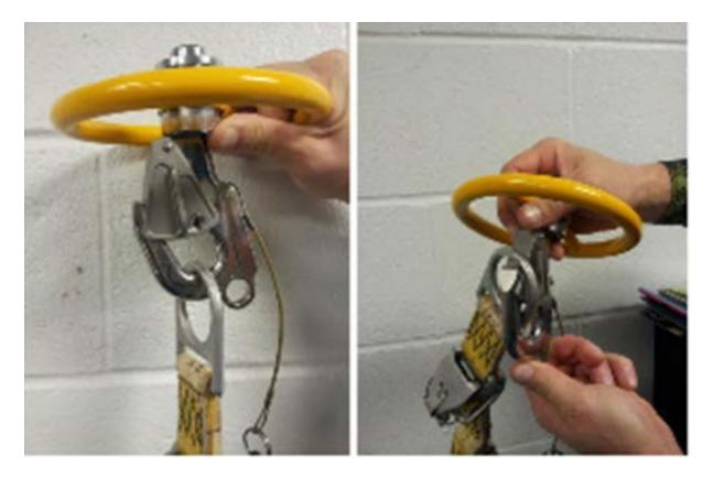
The investigation is focusing on technical causes, specifically a phenomena known as dynamic rollout, in which the rescue harness connecting D-ring can misalign with the hoist hook and allow the D-ring to disconnect. A Flight Safety *Flash* bulletin was immediately sent to all RCAF hoist users to identify this hazard.
