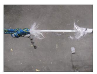
PMI 8mm accessory cord on 11mm EZ Bend, testing prusik behavior during slow pull. Six of 24 prusiks caused mantle failure as seen in the photo. The other 18 prusiks broke at the single cord strand strength of 15.46 kN. Photo by Thomas Evans.
