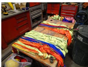
Seen here, 1,260 feet of old & retired webbing (donated by Seattle Mountain Rescue and the Southern Arizona Rescue Association), tied into slings for Wrap-3-Pull-2 and basket hitch anchor testing. After testing new and old webbing with knots in the anchor limbs, we have learned that the screw link is the weak spot for both anchor types (where webbing is most compressed). Photo by Sarah Truebe.
