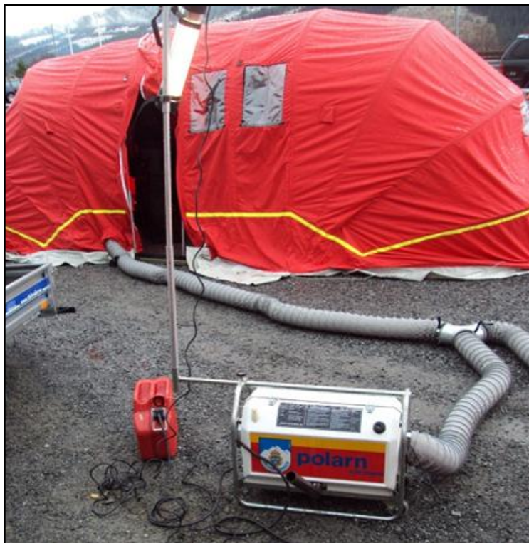
Emergency shelter with portable diesel heater and lighting. Used by rescue personnel during motor vehicles accidents requiring extrication. Due to extreme cold temperatures, shelter is deployed over a vehicle at an accident scene to provide instant shelter and heat during patient removal. Photo by K. Phillips.
