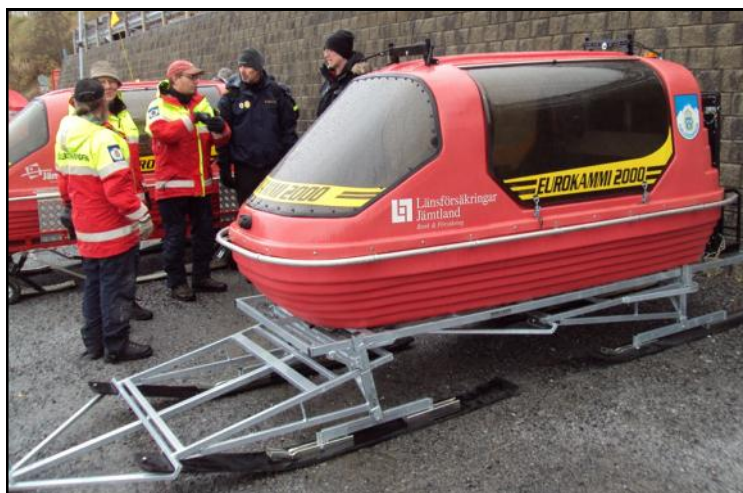
Over-snow patient transport trailer for use with snowmobile. Large size permits transport of patient and care provider side-by-side. Alcohol heater provides heat source during transports. Photo by K. Phillips.
