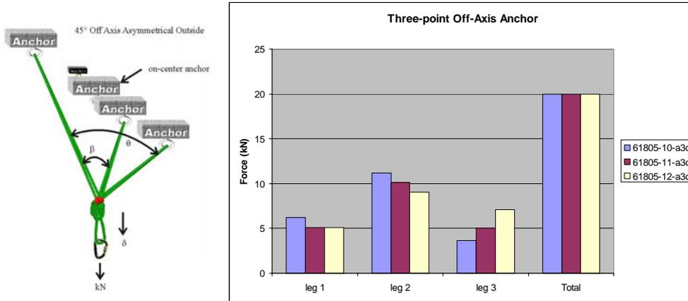
**Figure 10 and Figure 11:** Geometry and measured leg tension in three different test of three-point off-axis asymmetrical off-axis outside ( $\beta \neq \theta/2$ ) anchor.
