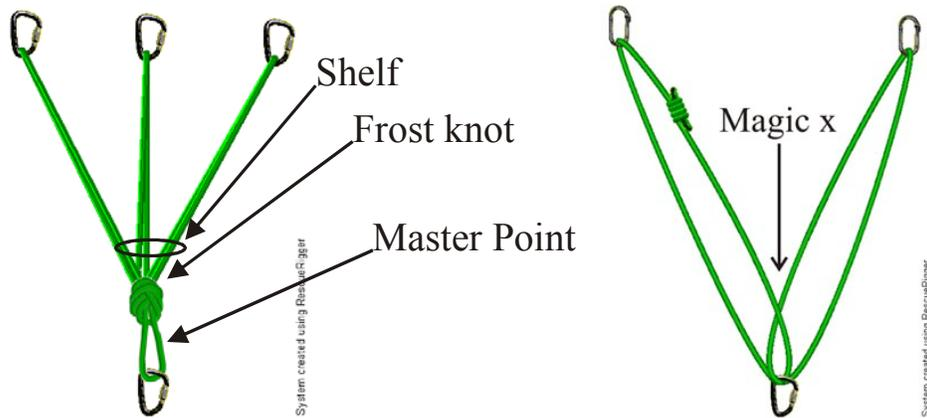
**Figure 1:** (left) A cordalette used in tying a 3 point symmetrical pre-equalized anchor; (right) an “equalized” or “Magic x”, shown here with only two points for clarity.
