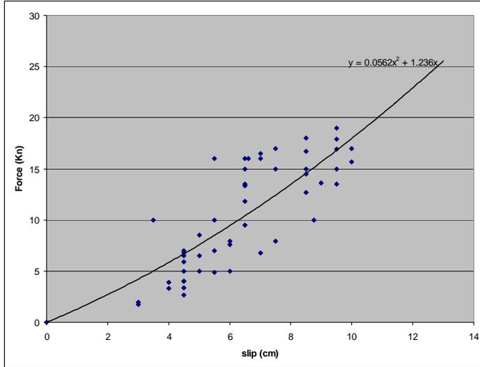
**Figure 22:** Knot slip as a function of leg tension.
