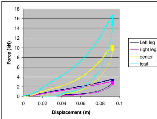
**Figure 7:** Force displacement relation for a typical symmetric, three-point anchor.
