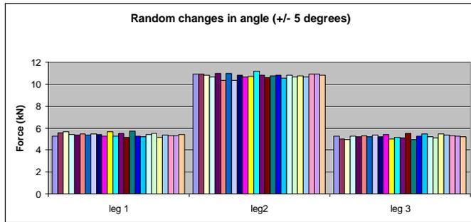
**Figure 25:** Effects on leg forces for a 3-point symmetric system from random changes of +/- 5 degrees in angle.
