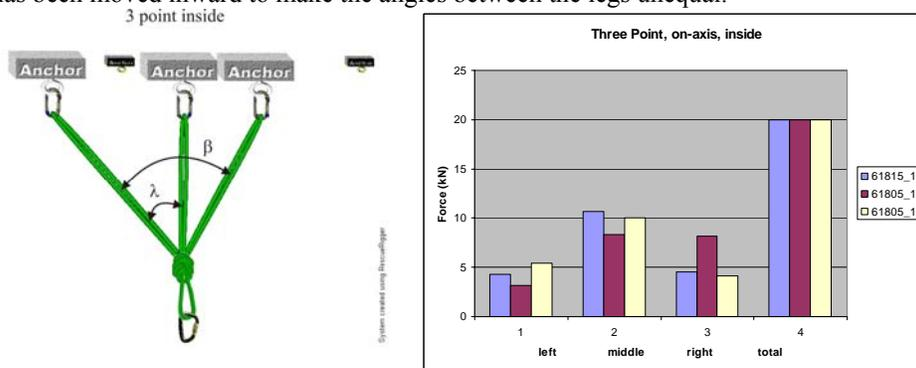
**Figure 5 and Figure 6:** Geometry and Measured force from three tests of a three point on-axis anchor with one leg moved to the inside.
