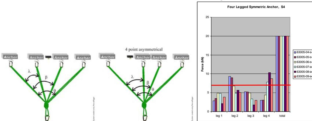
Figure 15, Figure 16, and Figure 17: Geometry and measured forces in a symmetric four-point anchor system. Geometry: symmetric (left) and asymmetric (right) 4-point anchor. The horizontal red line indicates a 7 kN load.
