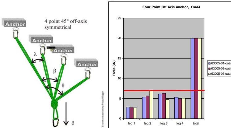
**Figure 18 and Figure 19:** Geometry and force distribution for off-axis four-point anchor system. The horizontal red line indicates a 7 kN load.
