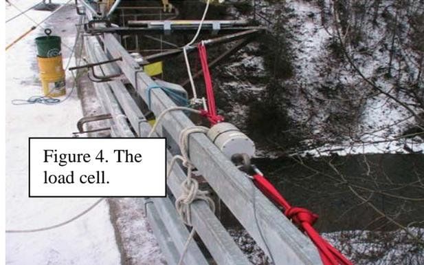
Figure 4. The load cell.
