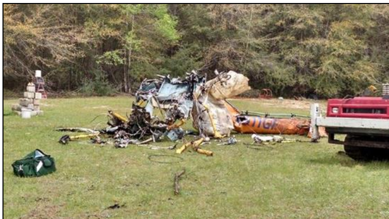
The wreckage was heavily fragmented with only the aft fuselage being generally recognizable.
