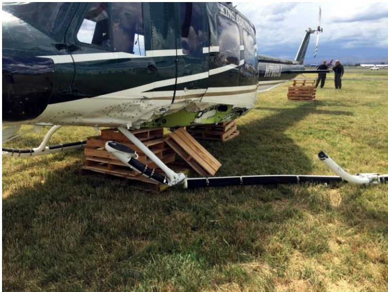
Damage to the King County Sheriff's helicopter sustained during contact with the ground. Pallets were arranged at a local airport to allow for a safe landing with damaged skid.
