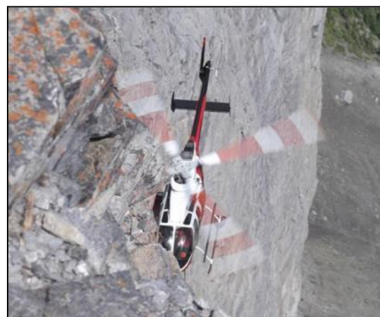
Moments after this photograph was taken, this helicopter's main rotor blades struck the rock at the 3 o'clock position during an attempt to insert a rescuer on a longline. There were no injuries, but the aircraft suffered significant damage.
