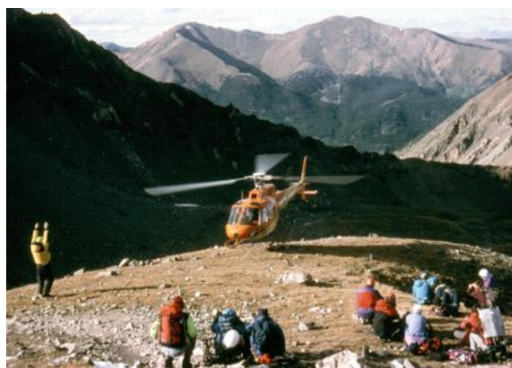
The ideal helispot is a flat strip 100 feet wide and 300 feet long (roughly the size of a football field). Photo: Dave Bathke
