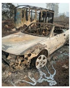
Car and Melted Aluminun Wheels
