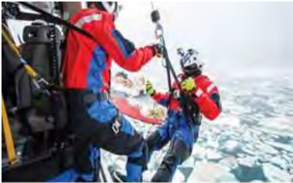
A hoist operation includes a raising and lowering mechanism on the side of the aircraft
