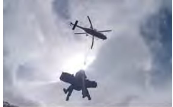
In a short-haul operation, rescuers and subjects are suspended on a fixed line.
